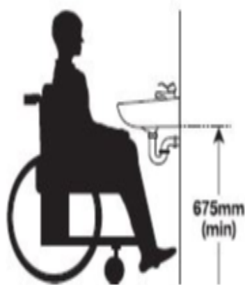
Figure 4. Wheelchair accessible basin
